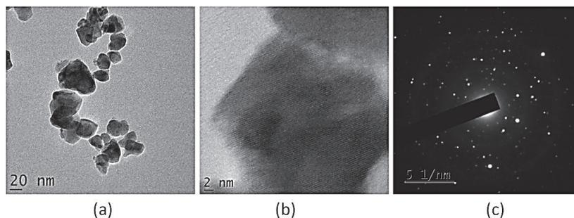
FIGURE 3. (a) Bright field image, (b) HR-TEM image and (c) SAED of NiWO<sub>4</sub> nanoparticles
