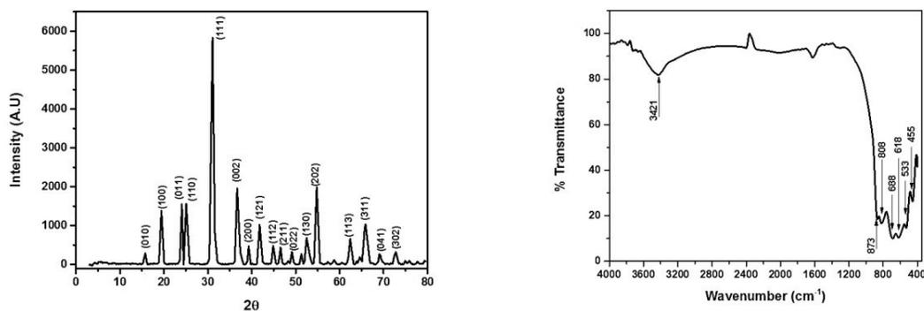
FIGURE 1. X-Ray diffraction patterns of NiWO<sub>4</sub> sample. FIGURE 2. FTIR spectrum of NiWO<sub>4</sub> sample
