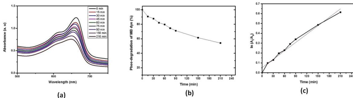
FIGURE 5. (a) Absorption spectra, (b) percentage degradation of MB with NiWO<sub>4</sub> and (c) linear plots of photo-degradation of MB with the NiWO<sub>4</sub>
