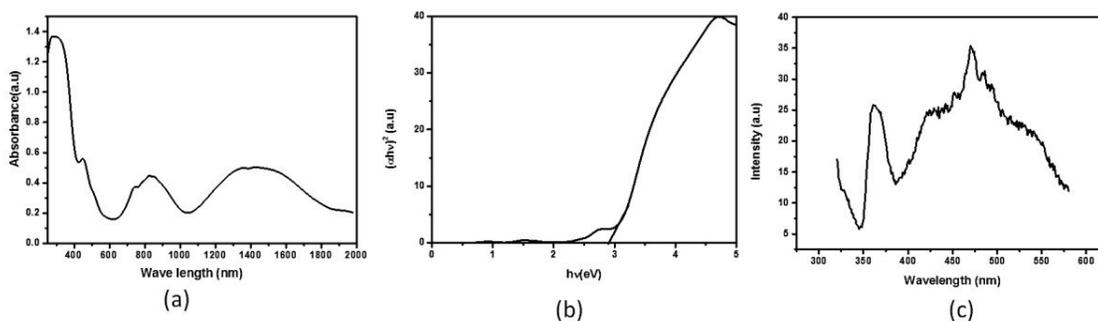
FIGURE 4. (a) Absorbance spectrum of NiWO<sub>4</sub> sample (b) Graph of  $(ahv)^2$  vs.  $h\nu$  for NiWO<sub>4</sub> sample (c) PL spectrum of NiWO<sub>4</sub> nanoparticle
