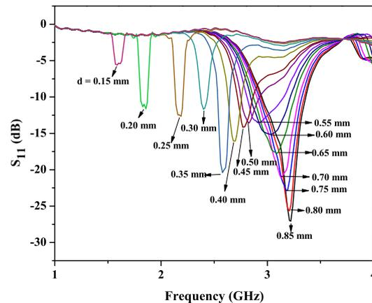
Fig. 3: The  $S_{11}$  characteristics of the BCSR loaded monopole patch antenna at different interplanar distances,  $d$ .
