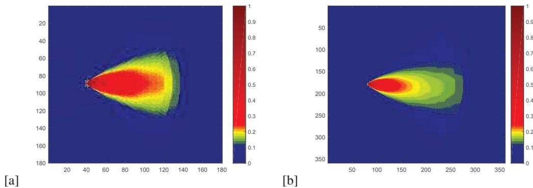
Fig. 3: Radiated electric field distribution near the ENG corner reflector antenna using standard FDTD for discretization parameter (a)  $N=8$  and (b)  $N=16$
