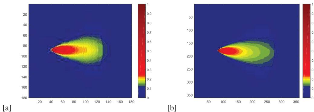
Fig. 2: Radiated electric field distribution near the ENG corner reflector antenna using NS-FDTD for discretization parameter (a)  $N=8$  and (b)  $N=16$
